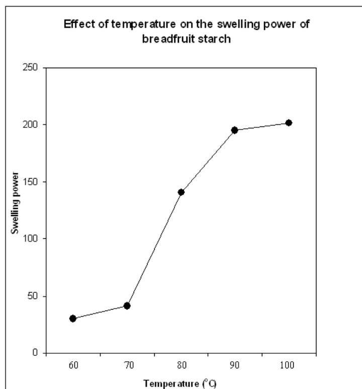
Figure 2. Effect of temperature on the swelling power of breadfruit starch
