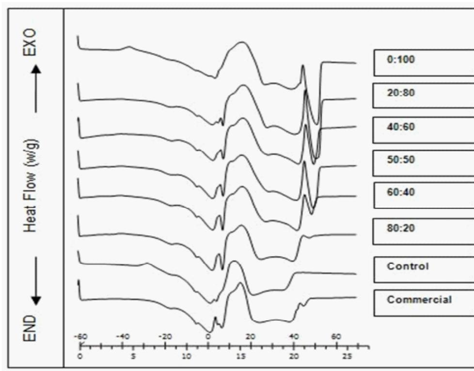
**Figure 4.** The differential scanning calorimetry heating curves of different types of shortenings based on the RBD palm oil/palm stearin blends and commercial shortening
