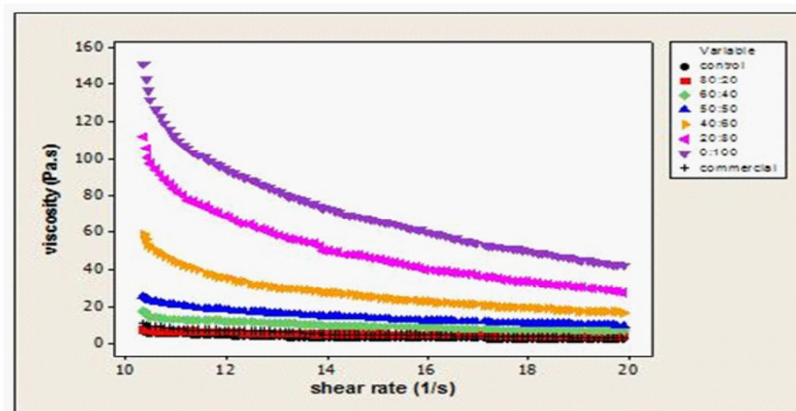
**Figure 1.** Variation of the viscosities (Pa.s) for the different types of RBD palm oil/ palm stearin and commercial shortenings, as a function of shear rate (1/s)
