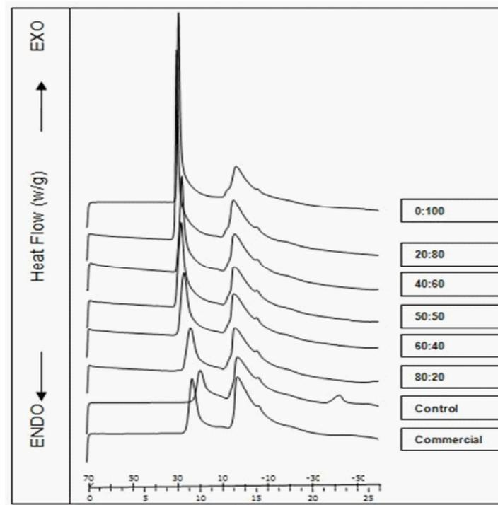
**Figure 3.** Differential scanning calorimetry cooling curves of different types of shortenings based on RBD palm oil/palm stearin blends and commercial shortening
