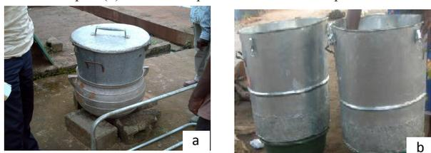
**Figure 3.** Improved equipment (a) General shape of the improved parboiler (b) The steaming vat
