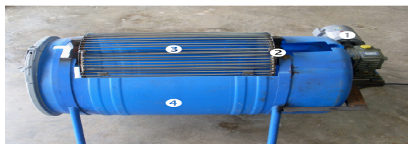
Figure 1. Lab-scale ginger washer/peeler: 1) motor, 2) water tank, 3) rolling vessel and 4) stainless steel grates
