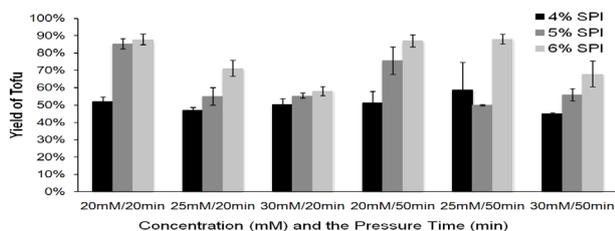
Figure 3. Impact of SPI (4%, 5%, 6%), GDL (20 mM, 25 mM, 30 mM) and pressuring time (20 min and 50 min) on the yield of the silken tofu
