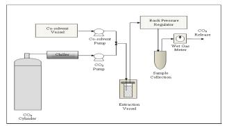
Figure 2. A schematic design of the supercritical fluid extraction (SFE) unit
