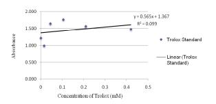
Figure 1. Antioxidant analysis by FRAP method shows the absorbance reading for different concentrations. By using equation of trolox standard, antioxidant concentration,  $(mM) = [(y - 1.3676) / 0.5653] \times 1 \text{ mg/mL}$
