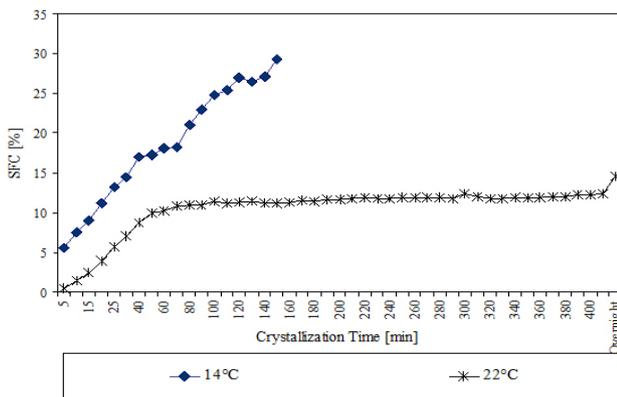
Figure 8. Solid fat content (SFC) [%] of RBDPO crystallized for 90 min at 14 and 22°C
