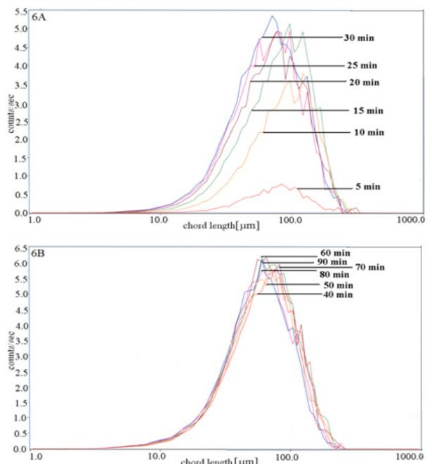
Figure 6. Chord length [ $\mu\text{m}$ ] distribution of RBDPO crystallized at  $22^\circ\text{C}$  for 5 to 30min (A) and 40 to 90min (B) (Sq wt)
