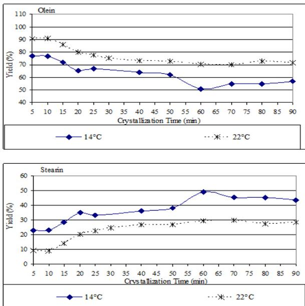
Figure 9. Yield of oleins and stearins during the 90 min crystallization of RBDPO at 14 and 22°C
