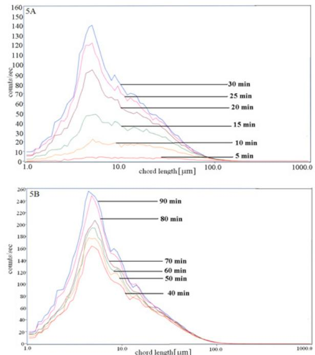
Figure 5. Chord length [ $\mu\text{m}$ ] distribution of RBDPO crystallized at  $22^\circ\text{C}$  for 5 to 30min (A) and 40 to 90min (B) (1/Lth wt)
