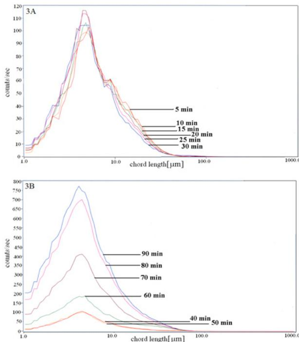
Figure 3. Chord length [ $\mu\text{m}$ ] distribution of RBDPO crystallized at  $14^\circ\text{C}$  for 5 to 30min (A) and 40 to 90 min (B) (1/Lth wt)
