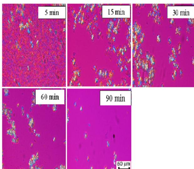
Figure 1. Light microscope photo of crystals formed during 5, 15, 30, 60 and 90 min crystallization of RBDPO at 14°C
