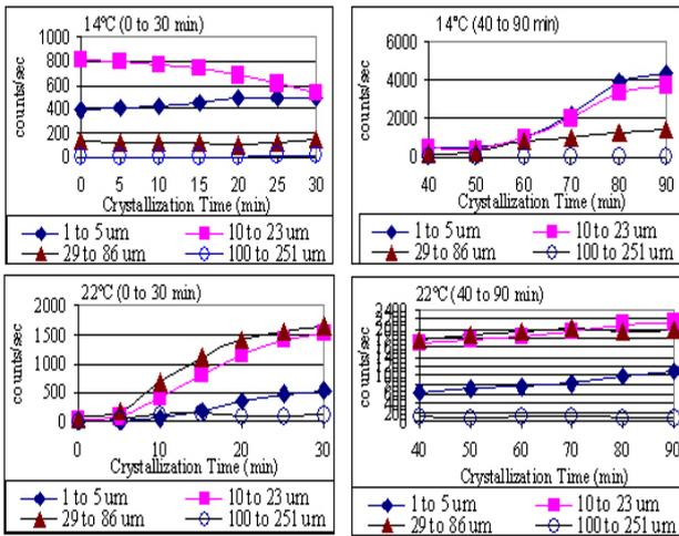
Figure 7. Crystal population [counts/sec] in RBDPO slurries during 0 to 30 min and 40 to 90 min crystallization at 14 and 22°C
