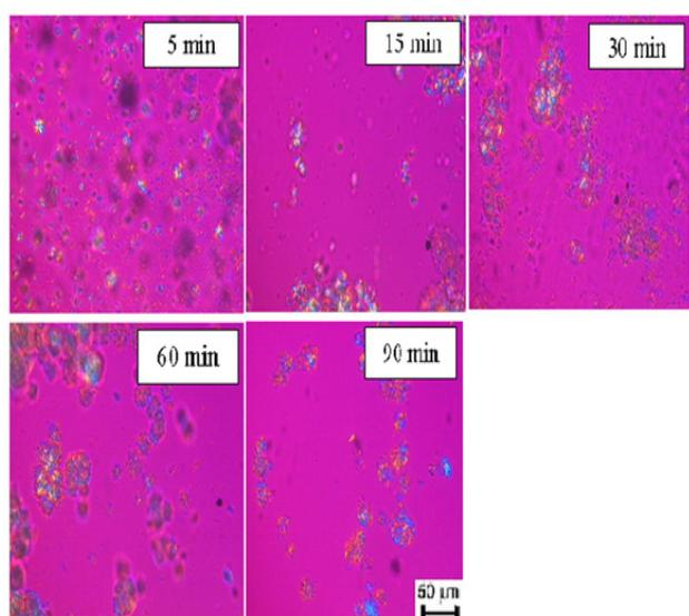
Figure 2. Light microscope photo of crystals formed during 5, 15, 30, 60 and 90 min crystallization of RBDPO at 22°C
