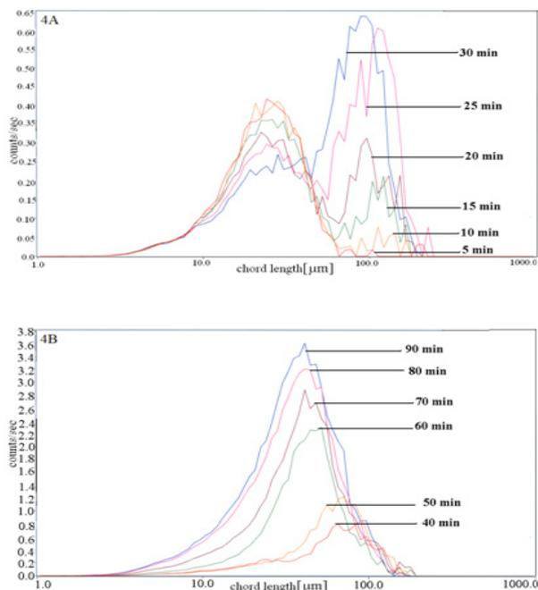
Figure 4. Chord length [ $\mu\text{m}$ ] distribution of RBDPO crystallized at  $14^\circ\text{C}$  for 5 to 30min (A) and 40 to 90min (B) (Sq wt)
