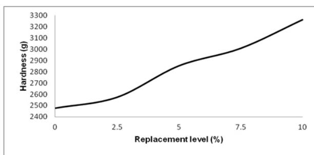
Figure 1. Effect of replacement level of refined wheat flour with pumpkin powder on hardness of biscuit.
