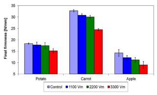
Figure 2. Final firmness vs applied electric filed strength.
