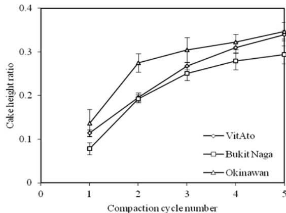
Figure 6. Caking height ratio to compaction cycle number of sweet potato flours
