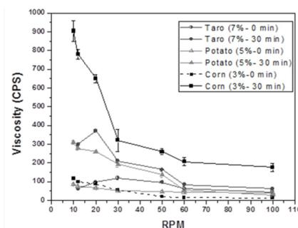
Figure 2. Viscosity (cps) of suspensions of native and modified OPT-120°C 30 min 5% w/w potato starch, 3% w/w corn starch and 7% w/w taro starch.
