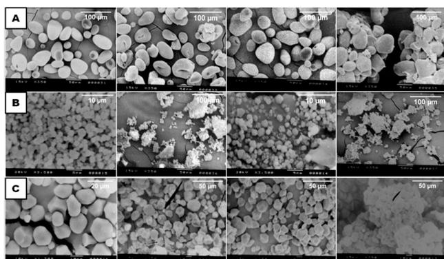
Figure 1. SEM of (A) potato starch, (B) taro starch, and (C) corn starch in its native, OPT-120°C-30 min, acetylated and cross-linked form (left to right).
