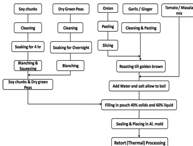
Figure 1. Flow chart for preparation and retort processing of soya peas curry
