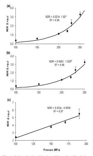
Figure 2. Inactivation kinetics of *Lactobacillus helveticus* (a), *Listeria innocua* (b) and *Pseudomonas fluorecens* (c) inoculated in skimmed milk and processed by high pressure homogenization (n = 3)
