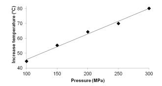
Figure 1. Temperature increases in skimmed milk samples processed by high pressure homogenization .Inlet temperature =  $23.0 \pm 1.0$ °C. Results shown are mean of triplicate trials on individual milk samples
