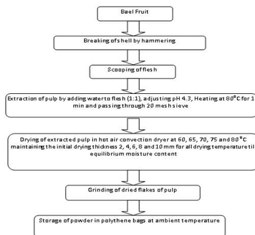
Figure 1. Flow chart of bael fruit pulp drying
