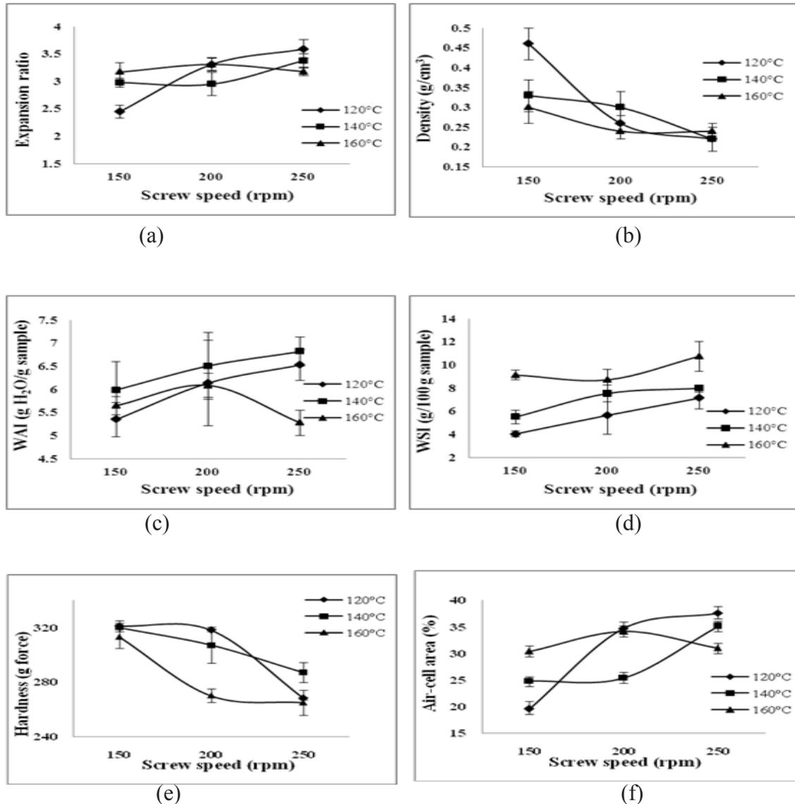
Figure 1. Effects of die zone temperature and screw speed on physicochemical properties of the extrudates
