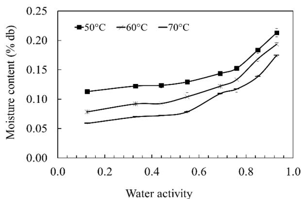
Figure 2. Moisture sorption isotherms of dried pumpkin powder at drying temperatures of 50, 60 and 70°C. Error bars represent standard deviation (SD)
