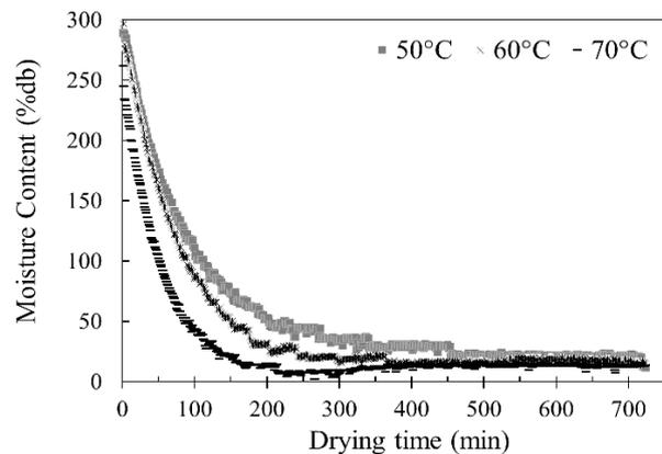
Figure 1. Moisture profile of pumpkin slices during drying at 50, 60 and 70°C
