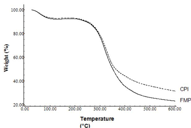
Figure 2. Thermogravimetric analysis of croaker protein isolate (CPI) and fish myofibrillar protein (FMP)
