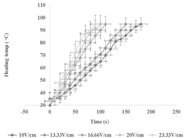
Figure 1. Time-temperature profile of watermelon juice ohmic heated at various voltage gradients
