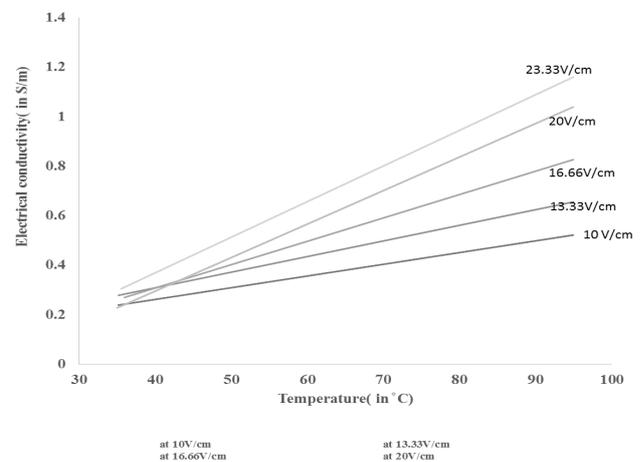
Figure 2. Electrical conductivity of watermelon juice with temperature at various voltage gradients
