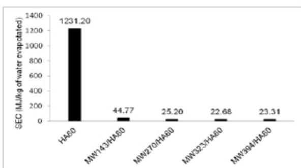
Figure 4. The specific energy consumption (SEC) of the silkworm pupae drying by microwave energy combined with hot air
