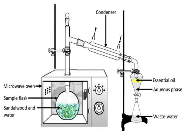
Figure 1. Schematic representation of the microwave-assisted extraction apparatus used in this study (Kusuma and Mahfud, 2016)
