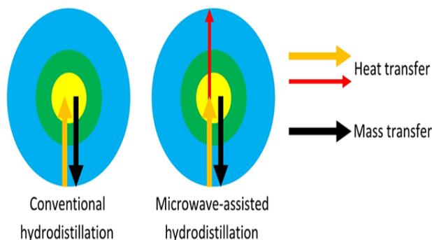
Figure 5. Heat and mass transfer mechanisms in microwave-assisted hydrodistillation and conventional hydrodistillation of sandalwood oil
