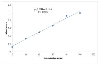
Figure 2. Standard calibration curve of gallic acid
