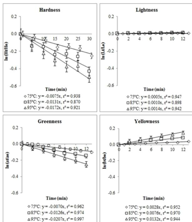
Figure 3. Effects of thermal processing on physical quality of tempe at 75°C, 85°C and 95°C.
