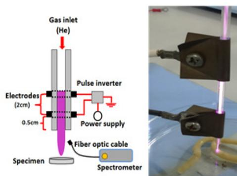
Figure 1. Plasma jet device and plasma when exposed to sample
