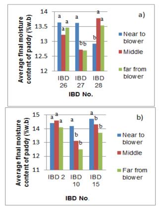
Figure 3. Comparison of average final moisture content obtained from different compartments in IBD (a) IADA KETARA (b) MADA. [The different letters indicate that the samples are statistically different according to Tukey HSD test (P<0.05)]
