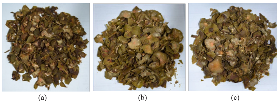
Figure 2. Appearance of batuan fruit pulps after drying at (a) 50°C, (b) 60°C, and (c) 70°C.
