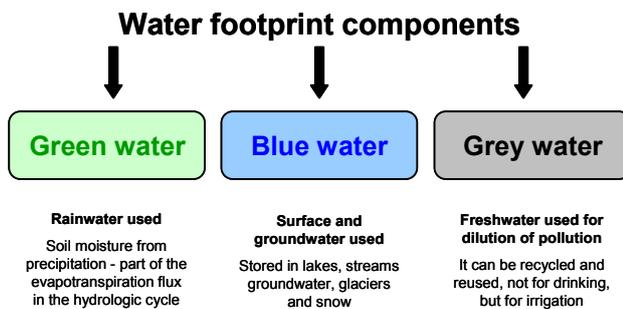
Figure 4. Water footprint components.
