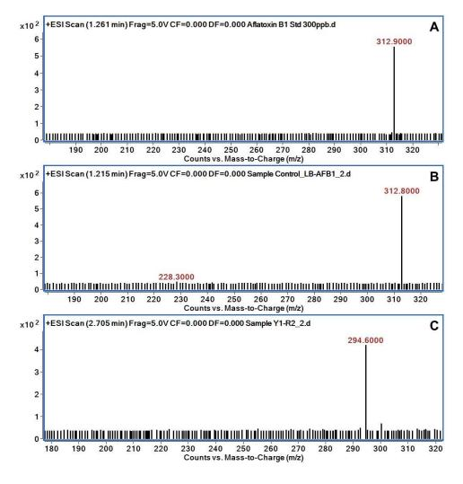
**Figure 1.** Mass spectra of (**A**) AFB<sub>1</sub> standard, (**B**) AFB<sub>1</sub> in LB broth (control), and (**C**) AFB<sub>1</sub> in LB broth after treatment with *B. subtilis* YGT1.
