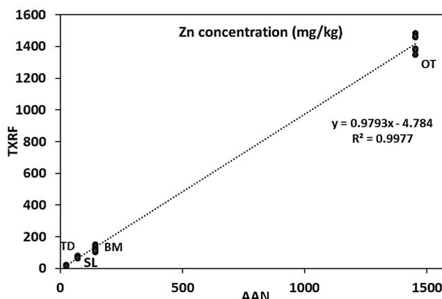
**Figure 5.** Comparison of Zn concentration resulting from TXRF and NAA ( $n = 6$  for each SRM TD, SL, BM, and OT). SL: spinach leaves, TD: typical diet, OT: oyster tissue, and BM: bovine muscle.
