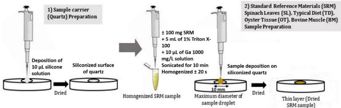
**Figure 3.** Preparation of thin-layer SRM (SL, TD, OT, and BM) sample by suspension method.
