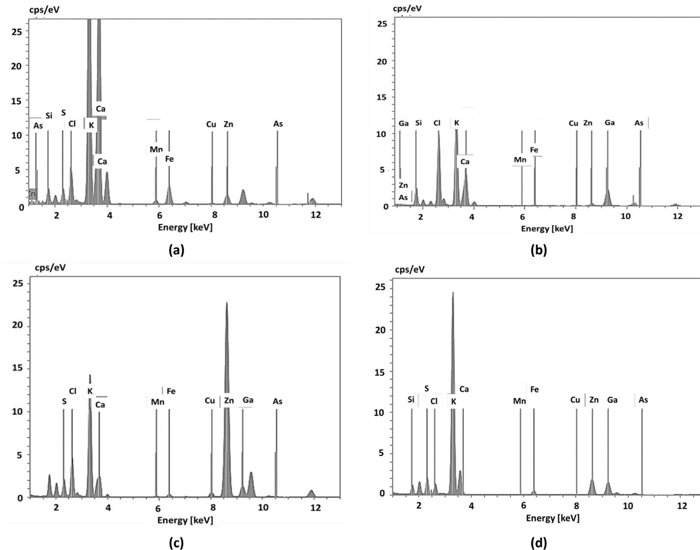
**Figure 4.** TXRF spectrum of (a) SRM NIST 1570a SL, (b) SRM NIST SRM 1548 TD, (c) SRM NIST 1566b OT, and (d) SRM NIST 8418 BM. SL: spinach leaves, TD: typical diet, OT: oyster tissue, and BM: bovine muscle. Each peak of elements represents the peak from k- $\alpha$ 1 lines.
