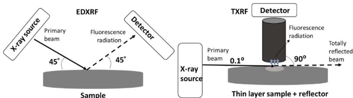
**Figure 1.** Conventional EDXRF (left) and TXRF (right) schemes.
