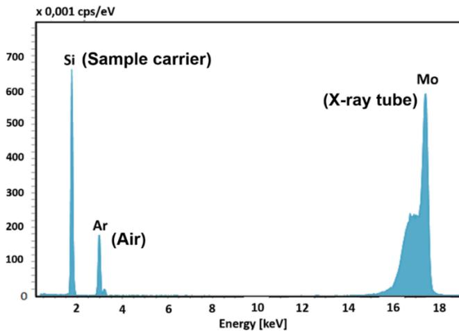
**Figure 2.** Spectrum of clean sample carrier. Si: sample carrier (quartz), Ar: air, and Mo: X-ray tube.
