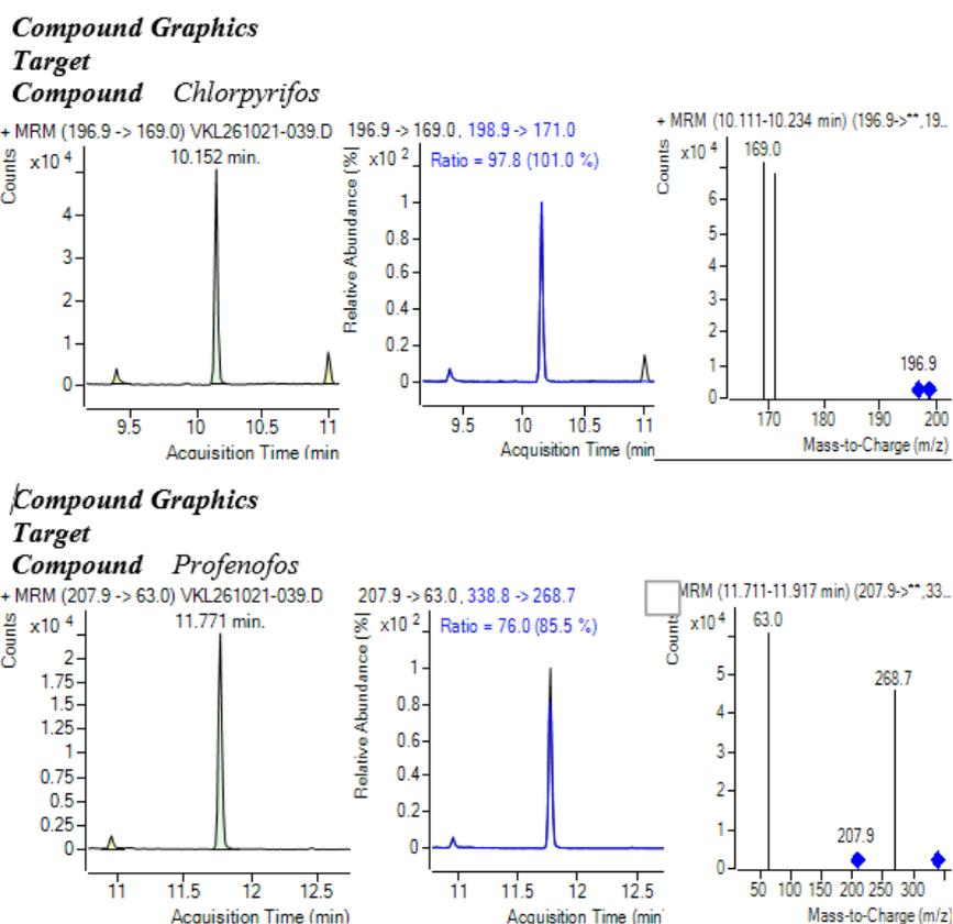
**Figure 1.** Chromatograms for chlorpyrifos and profenofos detected in kale sample by GC-MS/MS.
