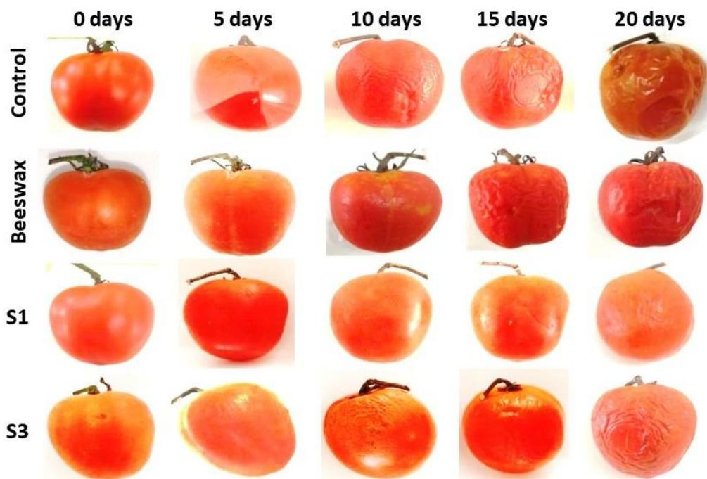
**Figure 2.** Fruit packaging performance of BC/glycerol/CMC/garlic (S1) and BC/garlic (S3). Uncoated tomato served as control, and beeswax-coated tomato as coating comparison.
