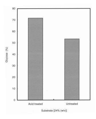
**Figure 6.** Production of glucose by RSDE using acid-treated and untreated sago starches. The reaction mixture containing 5 mL of 24% (w/v) acid-treated or untreated sago raw starches as substrate and 500 units of enzyme in a total reaction volume of 10 mL was carried out under optimum conditions (pH 5.5, 55°C) for 6 hrs.
