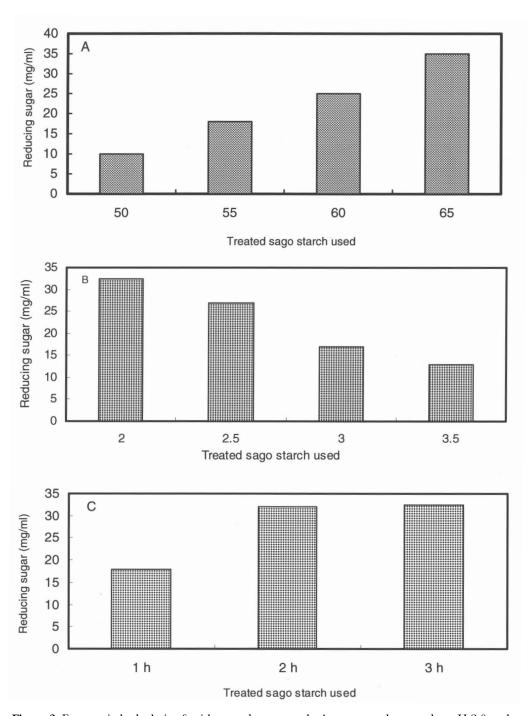
**Figure 3**. Enzymatic hydrolysis of acid treated sago starch. A: sago starch treated at pH 2.0 and temperature between 50-65°C for 2 hrs. B: sago starch treated at temperature 65°C and pH between 2.0-3.5 for 2 hrs. C: sago starch treated at pH 2.0, temperature 65°C for 1-3 hrs. The reaction mixtures containing 1 mL of 2% (w/v) acid-treated sago starch in 0.1M acetate buffer at pH 5.5 and 1 mL of RSDE was incubated at 55°C for 30 min.
