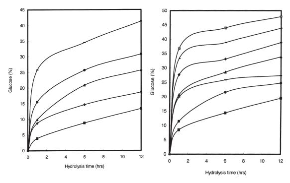
Figure 4: Enzymatic hydrolysis of acid treated sago starch (treated at pH 2.0, 65°C for 2 hrs) with RSDE at different concentrations. The reaction mixtures containing 1 mL of 2% (w/v) acid-treated sago starch dissolved in 0.1M acetate buffer at pH 5.5 with different concentrations of RSDE were incubated at 55°C for 30 min. Enzyme concentrations; ■: 20; ◆:40; ▲: 60; ●: 80; ■: 100 units/mL)
