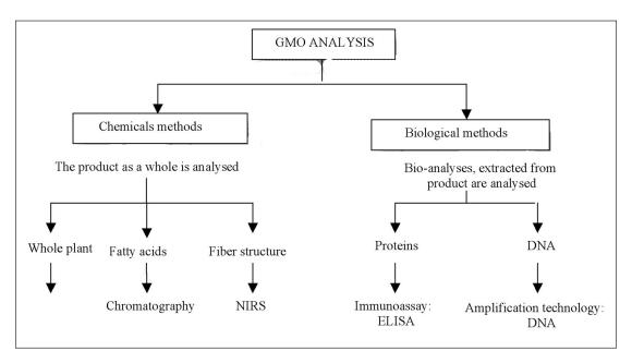
Figure 1: Classification of methods for GMO analysis (Adapted from Taverniers et al., 2004)
